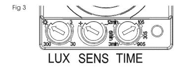
6. When you switch on the power, the light will be immediately turned on. It will turn off 10 sec later. Once the sensor detects presence from this point, it will operate as normal.
